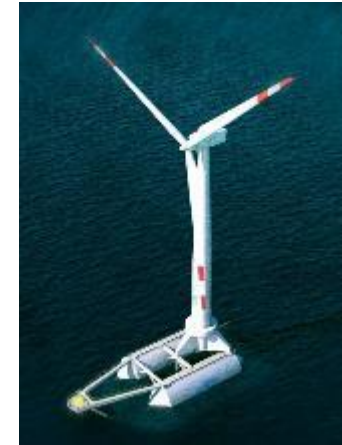
SAITEC – SATH: Barge floating Technology. Prototype 1:6 testing scheduled in 2020 (Santander)
