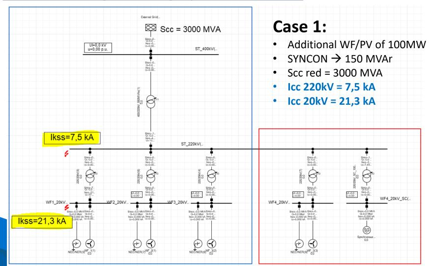
Simulation in existing node, adding a synchronous condenser:
